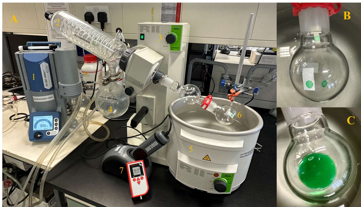
Figure 3.1. Images of the Rotavap system for barometric calibration of phosphorescent O_2 sensors. A. Main system components: 1-digital vacuum pump (with absorber of organic vapours); 2-condenser unit; 3-rotation motor assembly; 4-water/solvent collecting flask; 5-water bath; 6- sensor flask; 7-Optech and Firesting readers. B. Vacuum flask with different types of PtBP based sensors: O_2 Platinum sensor stickers (Mocon) attached to the neck (top), membrane with a solid-state sensor dot mounted in the bottom left part, and microparticle sensor (MPs) coating applied on the inner wall of the flask (right side); C. 100 mL flask with liquid NanO_2 -IR probe.
