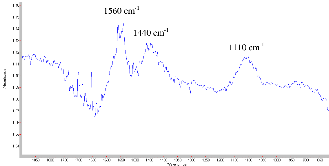
Figure 6.16: FTIR spectra of 0.1 wt% malonic and 1 wt% sulfuric acid aerosols with 300 sccm ammonia at 50 %RH.
