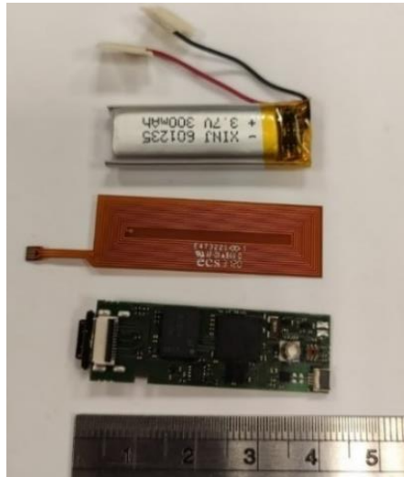
Figure 29 - From top to bottom, system components: battery, antenna, and PCB.
