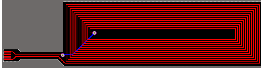
Figure 21 - Flexible PCB design for the antenna.
