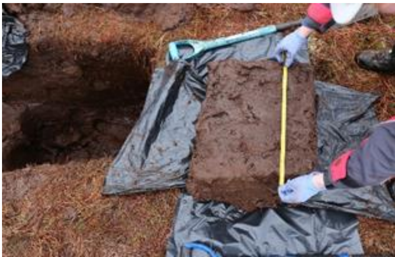
Figure 3-3: Undisturbed peat block sample excavated from a depth of 0.6–0.87 m below ground level in Location 1
