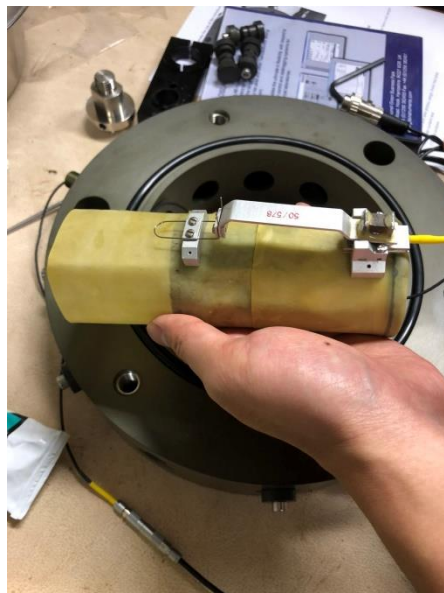
Figure 4-8: A specimen with a Hall effect sensor
