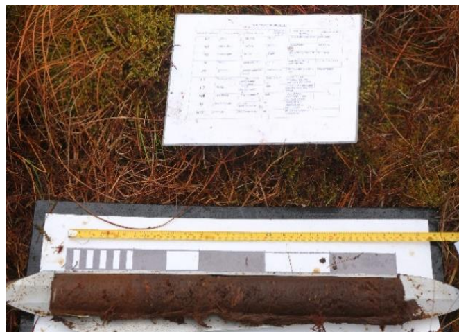
Figure 3-2: Field peat logging and classification using a Russian corer
