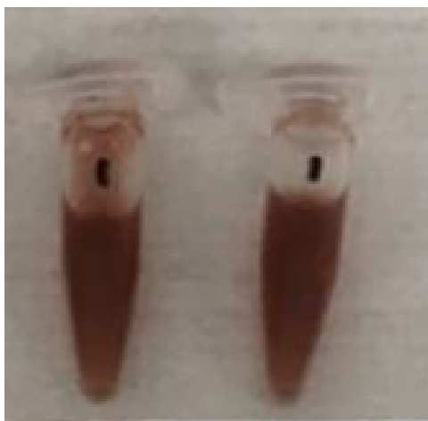
Figure S2: Given enough time, AgNO 3 and Gum Arabic would chemically react to form Ag-Gum Arabic nanoparticles.
