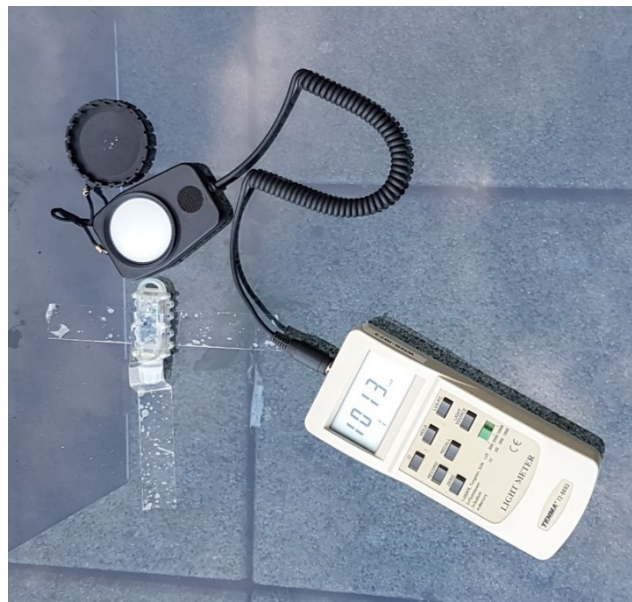
Figure 16. Light measurement calibration of AquaBit.
