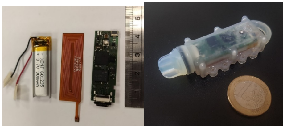
Figure 8. Final embedded system for seaweed monitoring before and after encapsulation for deployment.
