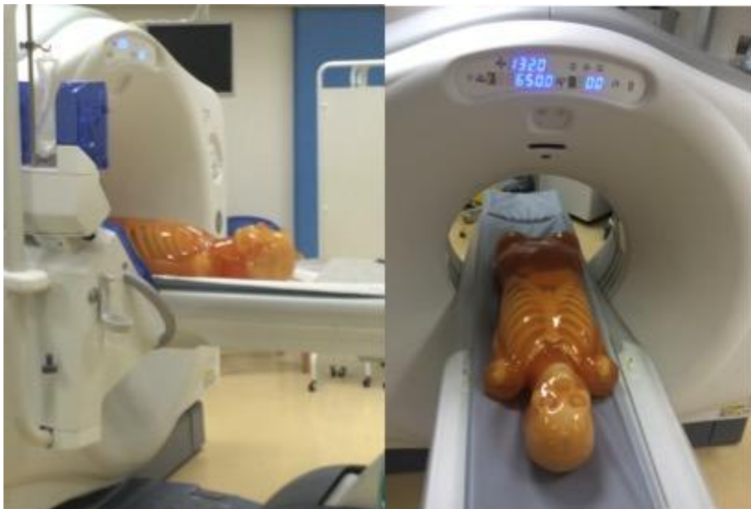
Figure 2.1: Kyoto anthropomorphic phantom positioning on the CT table. The phantom is placed supine and lateral and antero-posterior CT localiser radiographs are obtained.
