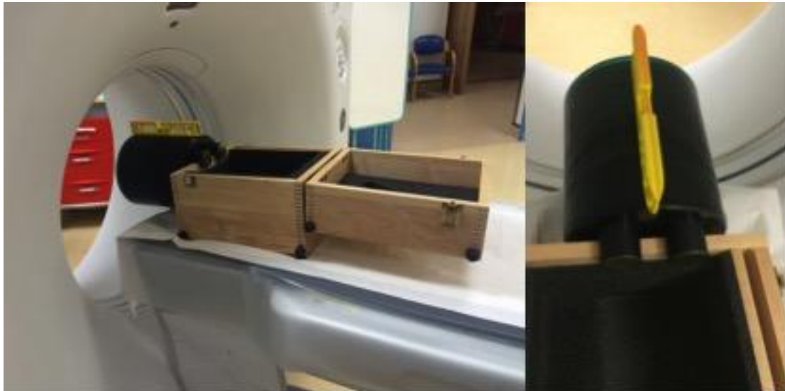
Figure 2.4: Photographs of Catphan 600 phantom in position on the CT table. The box is used to support the phantom with the CT gantry laser guides and spirit level used to align the phantom with the gantry isocentre.
