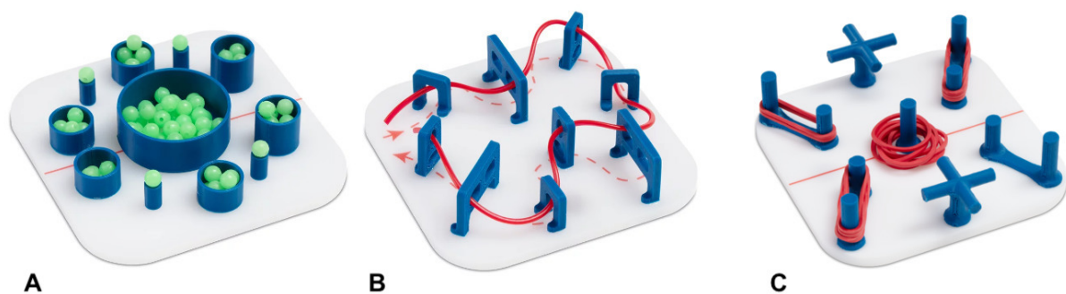
Figure 6.2: Bead transfer task (A), threading task (B) and band stretching task (C)
