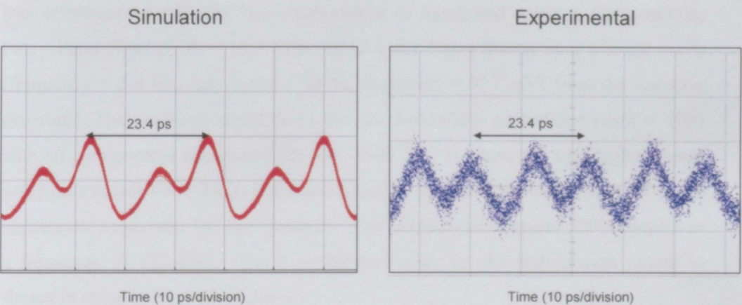
Figure 3.18. (a) Simulated and (b) Experimental scope traces for a seven channel phase locked optical comb
