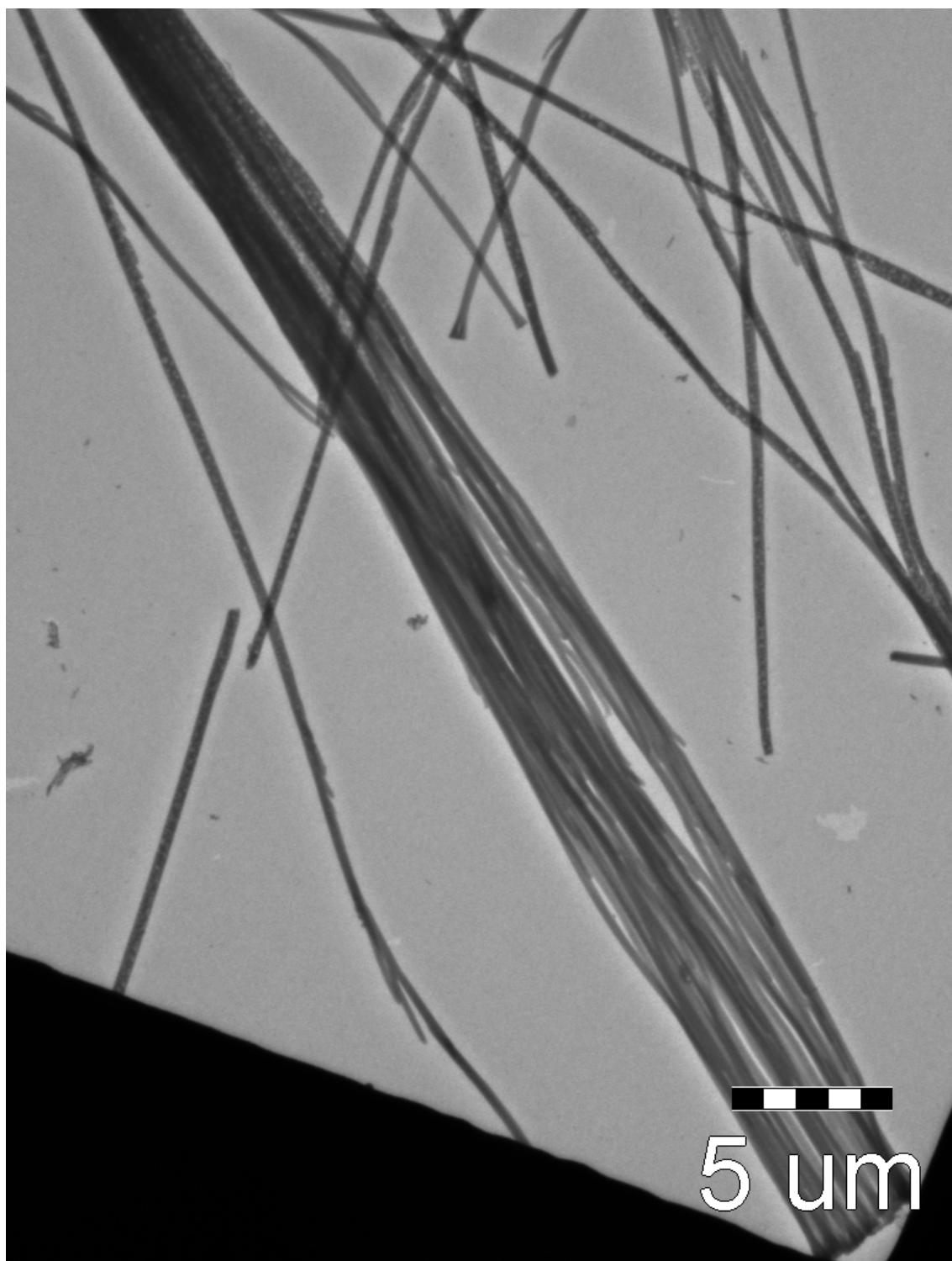
**S2** Low magnification TEM image of mesoporous carbon nanofibres released by dissolving AAO membranes in a 6M HCl solution. The Y-shaped branches and saw-shaped edges in some nanofibres vividly reflect the inner surface morphology of pore channels of AAO membranes
