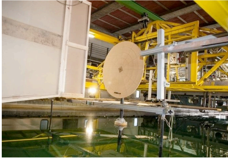
Figure 5 Wind generation on a drag disk during hybrid wind/wave device testing at INSEAN (taken from [28])
