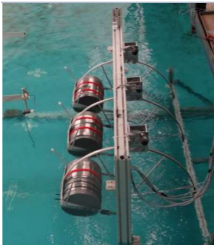
Figure 7: Model of scale1:30 WEC proposed for hybrid wind-wave device [40]
