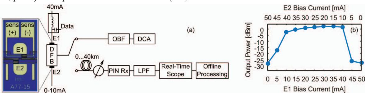
Fig. 1. (a) Experimental setup; (b) Output power as a function of different electrode current ratios for a constant total current of 50mA.
