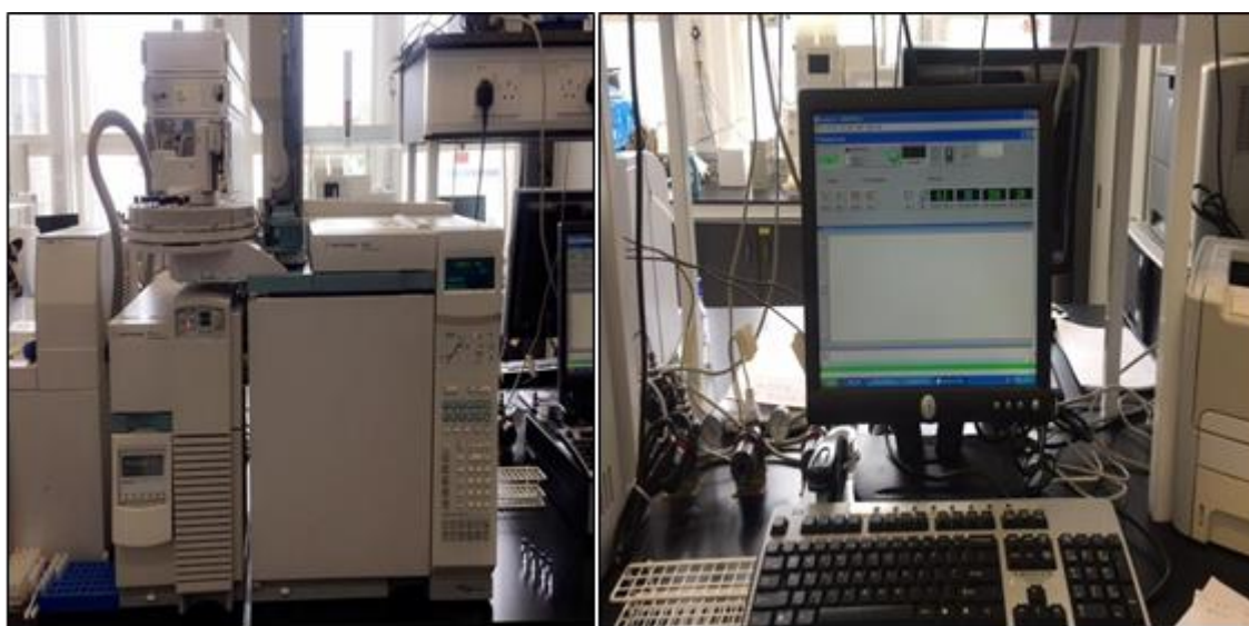
Figure 5.2 Agilent 6890/5973 gas chromatography-mass Spectrometry (GC-MS) instrument.
