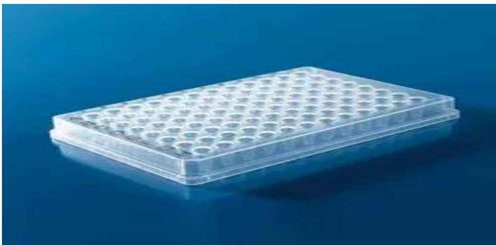
Figure 1.4 ELISA 96 well plate is made from clear polystyrene that is suitable for optical detection.
