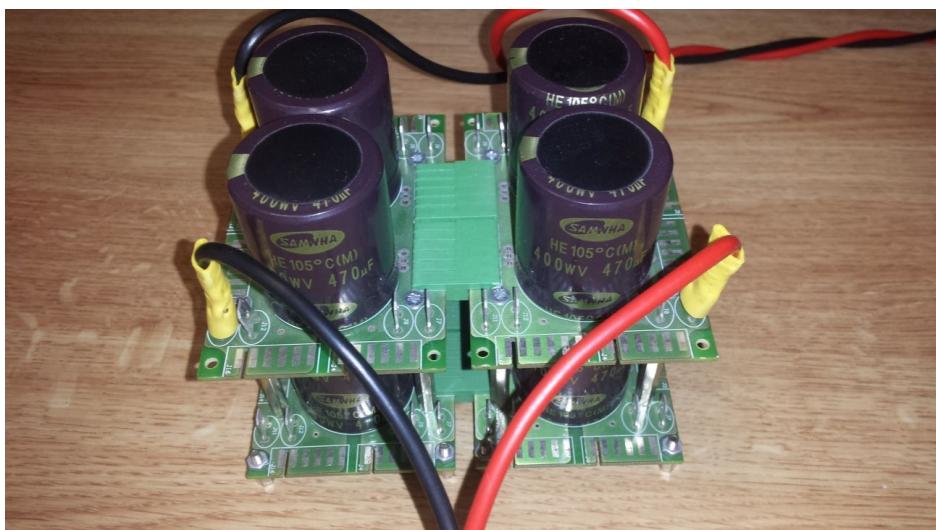
Figure 2.31. The converter output capacitor
