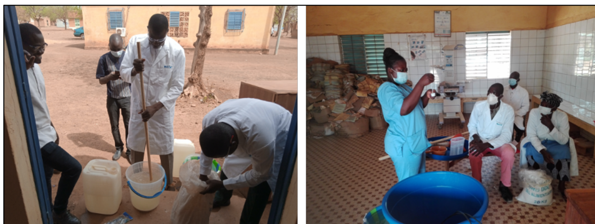
Figure 17. On the left: mixture of salty water for production. On the right: quality control of sodium hypochlorite produced (Antenna Foundation Archives).
