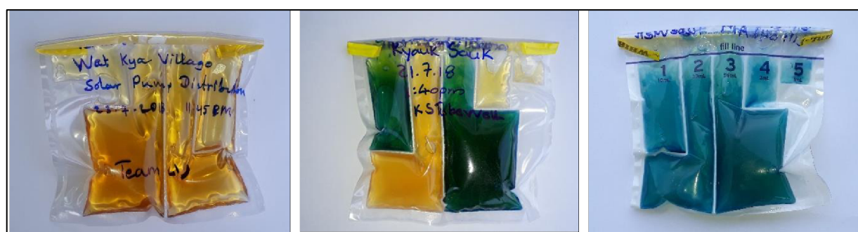
Figure 35. Chlorolimetric analysis for the detection of the bacteria Escherichia coli . (A) safe - (0 MPN/100ml), (B) intermediate risk (3.4 MPN/100 ml) and (C) Unsafe (over 100 MPN/100 ml).
