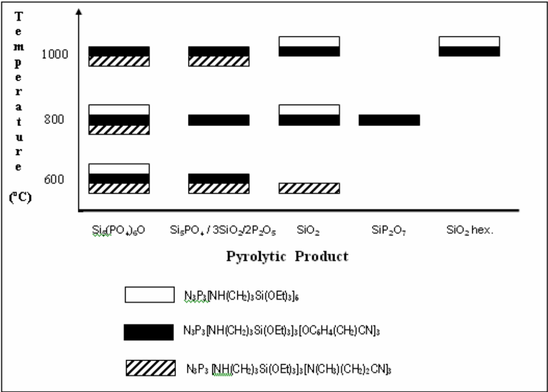
Scheme 3 Schematic representation of the distribution of products from pyrolysis of precursors (1), (2) and (3) at several temperatures.
