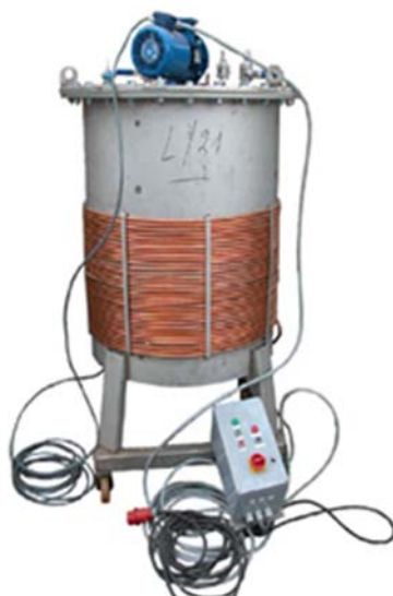
Figure 1.25: Custom-made reaction vessel (900 litres) [58]
