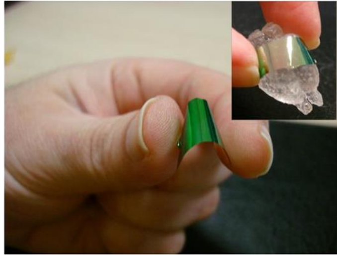
Figure 5.1: AlN deposited on flexible material for use in biomedical applications [72]
