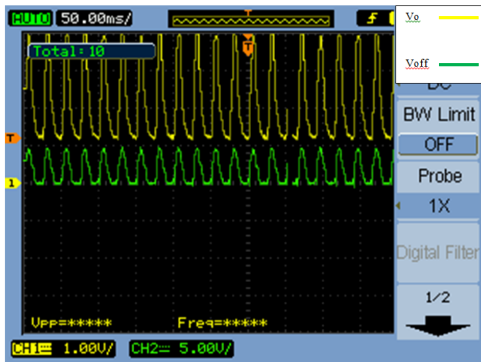
Figure 6.29: V_o (Yellow) and V_{off} (Green) from Bread-boarded Romani et al. Circuit, 1 output
