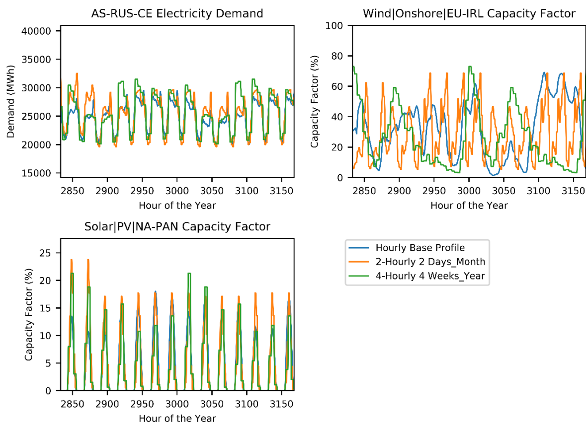
Figure D-6 Examples of sampling combinations for a variety of demand and VRES series. Examples are given for Asia - Central Russia (AS-RUS-CE), Europe - Ireland (EU-IRL) and North America - Panama (NA-PAN).
