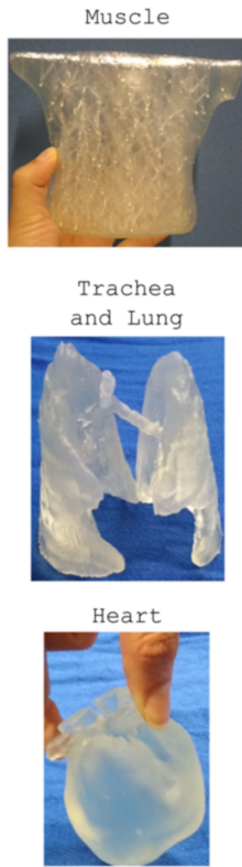
Figure 3.2. Resin 3D printed models of main organs, used to make the negative moulds of the anthropomorphic phantom from Paper III.
