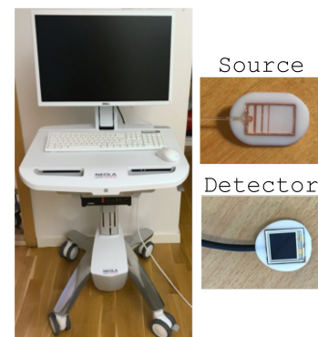
Figure 2.6. NEOLA-alpha 2, clinical research system for GASMAS measurements in lungs of newborns. The area of the diffuse light source is 1 \text{ cm}^2 with maximum output powers of 25 mW at 764 nm and 8 mW at 935 nm. The detector consists of a photodiode with a sensitive area of 1 \times 1 \text{ cm} . Both probes are attached to the infant's skin with a double sided medical tape.
