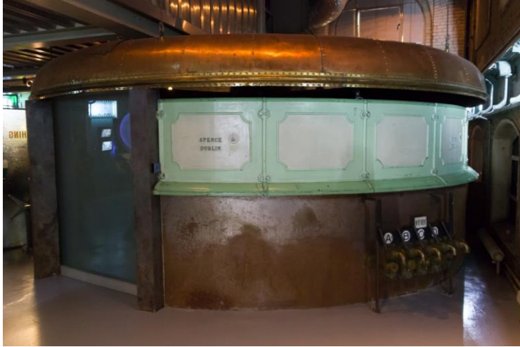
Plate 5.10. Cast-iron mash tun by Spence of Dublin. Guinness Storehouse, Dublin. The painted and panelled section of mash tun wall was visible above floor level when originally installed in the Brewery no. 2. The plain cast-iron section below was below floor level. Note the wort outlet pipes in the bottom right.
