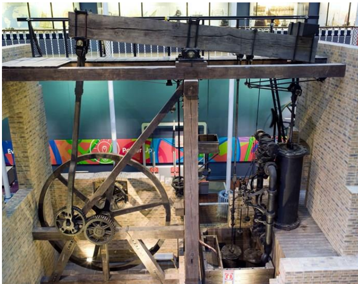
Plate 7.10. House-built Boulton and Watt beam engine at the National Museum of Scotland, Edinburgh. It was originally installed in Barclay's Brewery in London in 1786 and remained in use at the brewery until 1885. Watt's 'parallel motion' can be seen connecting the piston to the beam, on right. The 'sun and planet' gears can be seen on left.
