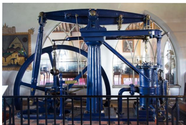
Plate 7.14 Two-column, independent beam engine. Originally installed at the St. Francis's Abbey Brewery, Kilkenny city. Now at the Straffan Steam Museum, county Kildare.
