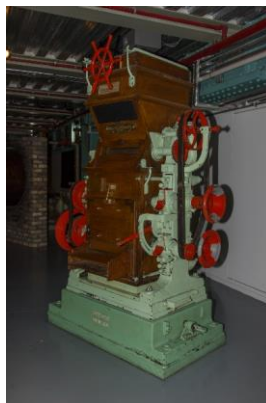
Plate 5.1. Ganz roller mill, produced in Budapest, Hungary. Guinness Storehouse, Dublin.
