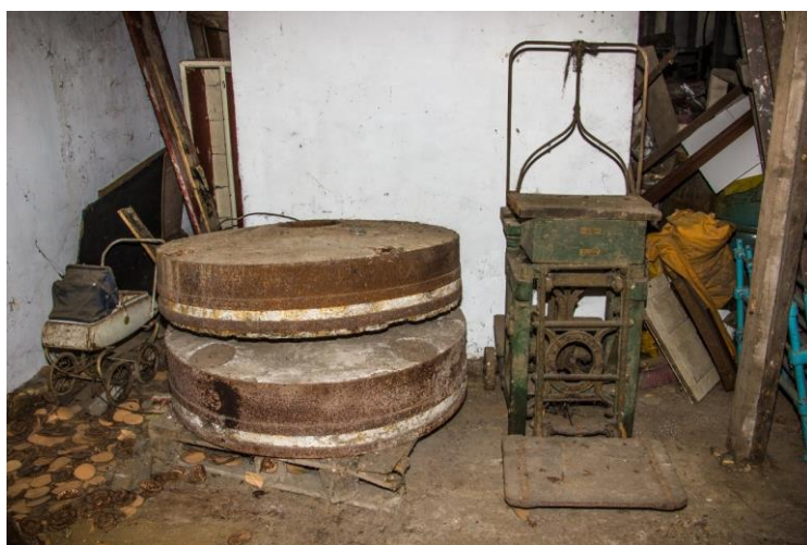
Plate 5.5. Millstones and Avery's grain weigher, the Mill Park Brewery, Enniscorthy.
