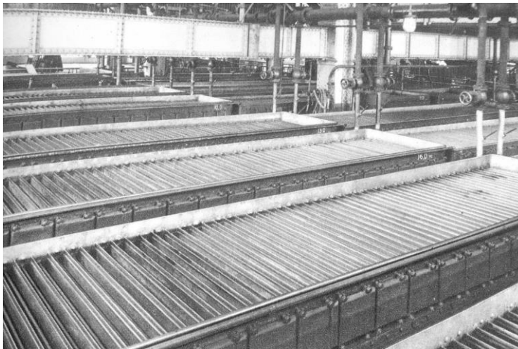
Plate 6.2. Horizontal refrigerators at Guinness, Dublin. Late-19th or early 20th century (anon. 1939).
