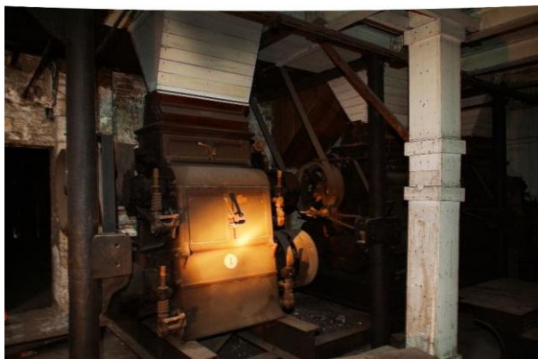
Plate 5.2. Roller mill no. 1, produced in Dresden, Germany. Malt-milling loft, Beamish and Crawford, Cork (courtesy Diarmuid Ó Drisceoil).
