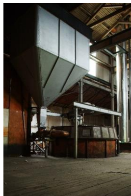
Plate 5.13. Mash tun, grist case and Steel's mashing machine, Beamish and Crawford, Cork. (courtesy Diarmuid Ó Drisceoil).
