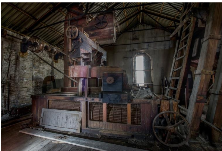
Plate 5.3. Rotary screening plant, Beamish and Crawford (courtesy Diarmuid Ó Drisceoil).
