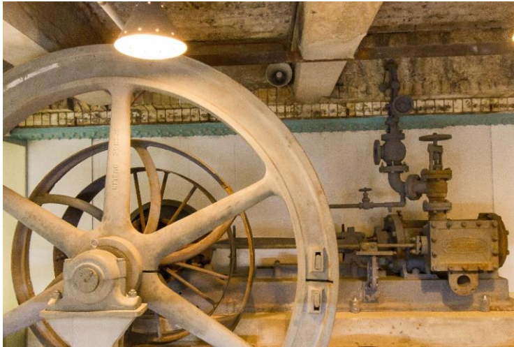
Plate 7.19. Horizontal non-condensing engine by Spence of Dublin. Installed in Guinness's Cooke's Lane maltings in c. 1896. Guinness Storehouse, Dublin.
