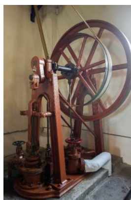
Plate 7.13. A-frame independent steam engine. Originally installed at the Watergate Brewery in Bandon, county Cork. Now at the Straffan Steam Museum, county Kildare.
