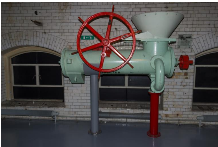
Plate 5.8. Painted cast-iron Steel's mashing machine, manufactured by Spence of Dublin. Guinness Storehouse, Dublin.
