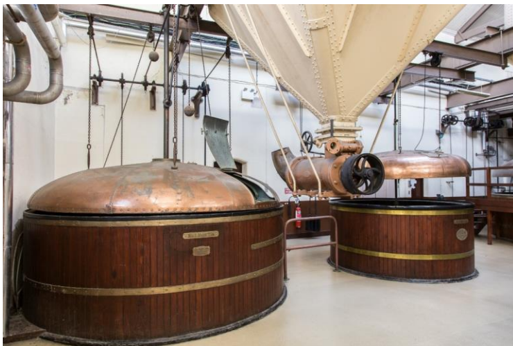
Plate 5.11. Mash tuns nos. 1 and 2, the St. Mary's Brewery, Waterford. Both mash tuns were fed by a single Steel's mashing machine, suspended from the ceiling between. Note the counterbalance chain and pulley system for lifting the copper lids.
