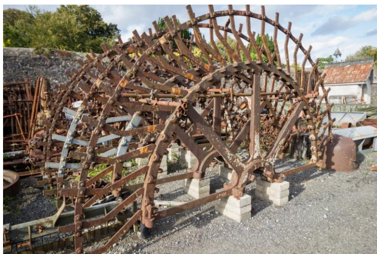
Plate 7.9. Cast-iron water wheel, originally from the St. Francis's Abbey Brewery, Kilkenny city. Stored, in two halves, at the Straffan Steam Museum, county Kildare.
