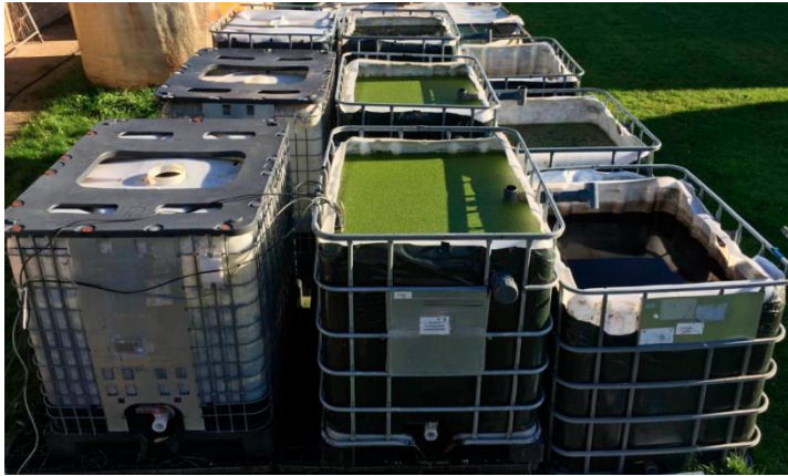
Figure 8: Experimental setup from (Devlamynck et al., 2021a). The IBC on the left is used for storage and mixing of the influent. It is pumped into the middle IBC where duckweed is cultivated. The lower IBC is filled with effluent by an overflow mechanism
