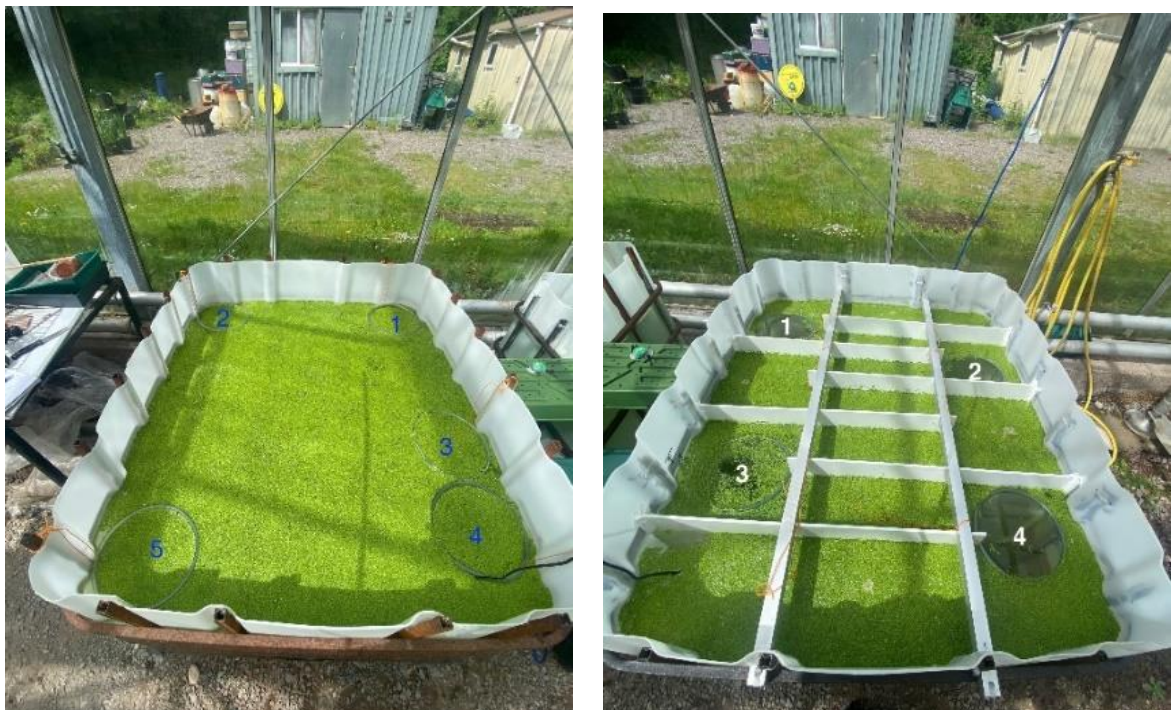
Figure 18: Overview of ring locations in each system a) system with no baffles, b) system with baffles
