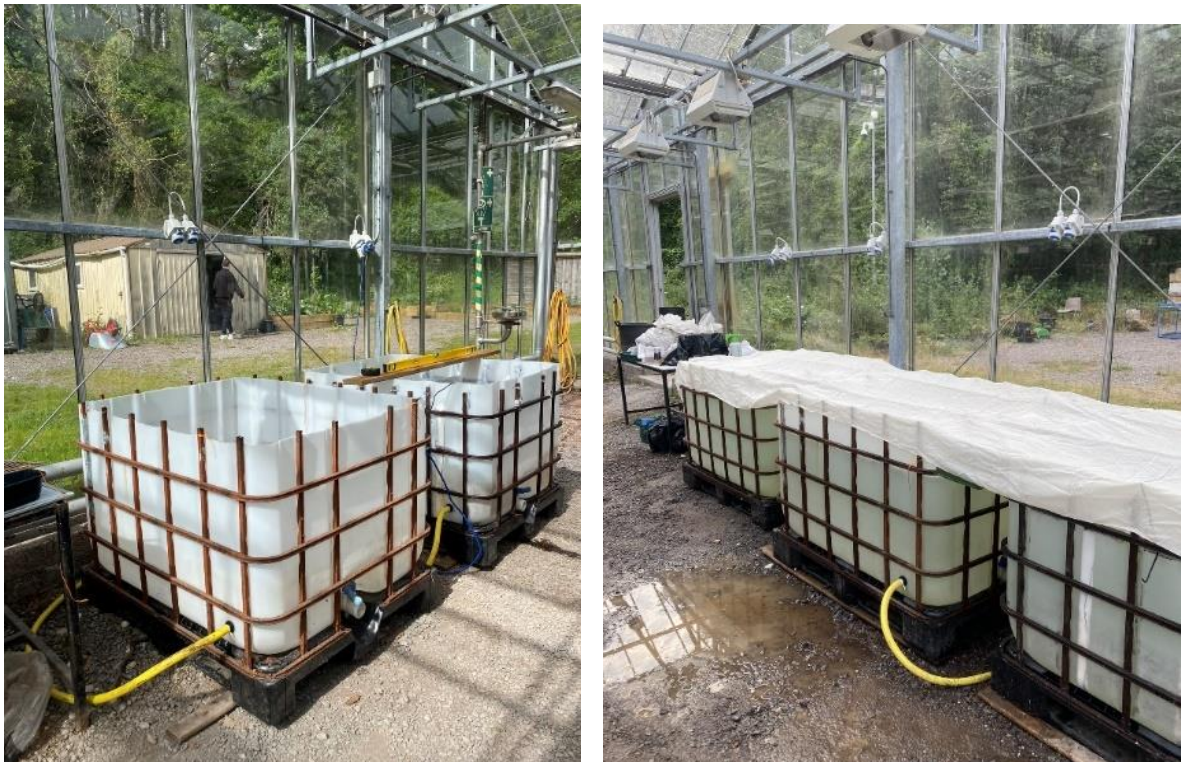
Figure 19: IBC setup in the glasshouse a) ensuring the IBCs are level b) muslin draped across the IBCs to reduce light intensity
