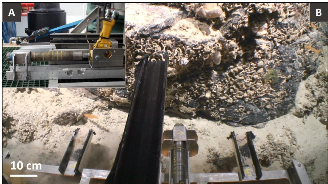
Figure 8: Hydraulic rockdrill mounted to the tool sled at the front of the Holland 1 ROV (A), and rockdrill sampling in action (B) on the seafloor (D26, approx. -1132 m).
