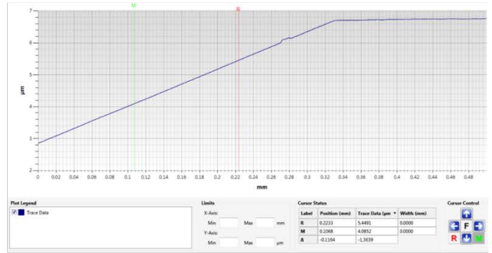
Figure S8 | Junction depth by bevel analysis. Bevel analysis of the p + surface region for buried junction depth. A) -- A staining solution is applied to the beveled surface plating the underlying nSi. B) – From the surface profiler the angle of \sin \theta = 0.0112 and the hypotenuse of 40.0 μm are determined for a calculated junction depth of 0.448 μm.
