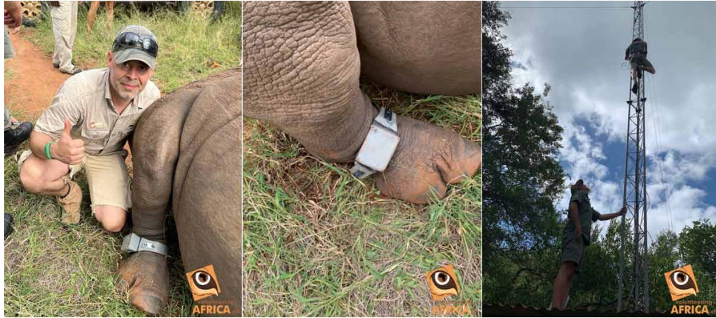
Figure 2.2: The LoRaWAN connected trackers get attached on collars which are then buckled onto rhino's legs [44]
