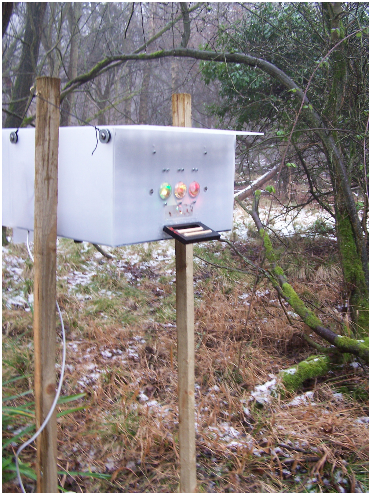
Fig 1. One of the portable operant devices installed in Wytham Woods, Oxford, UK. The weatherproof external casing is made of opaque Perspex, while the three response keys and the section of the front panel comprising the feeding hole are transparent. The perch (bottom of the front panel) is equipped with an antenna that relays information about the unique PIT-tag combination of marked individuals to the printed circuit board located within the device.
