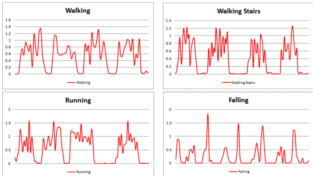
Figure 3: The thigh gyroscope signal of different activities
