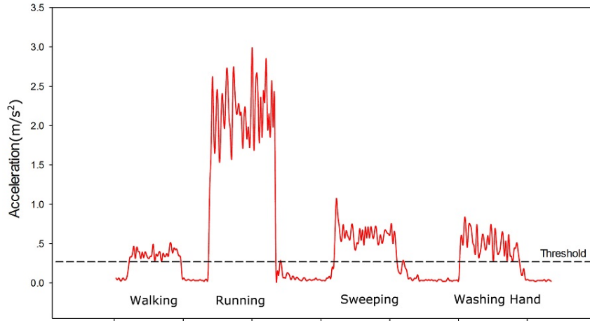
Figure 5.5: Standard Deviation threshold for trunk accelerometer signals
