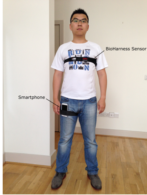
Figure 4.9: Activity recognition using smartphone associated BAN
