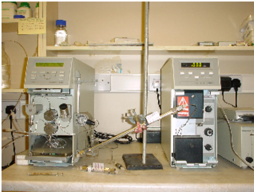
Fig 4.12 SE HPLC system: includes isocratic pumps (left), manual injection port (left of centre), guard column (on bench), separation column (centre) and UV detector (right).
