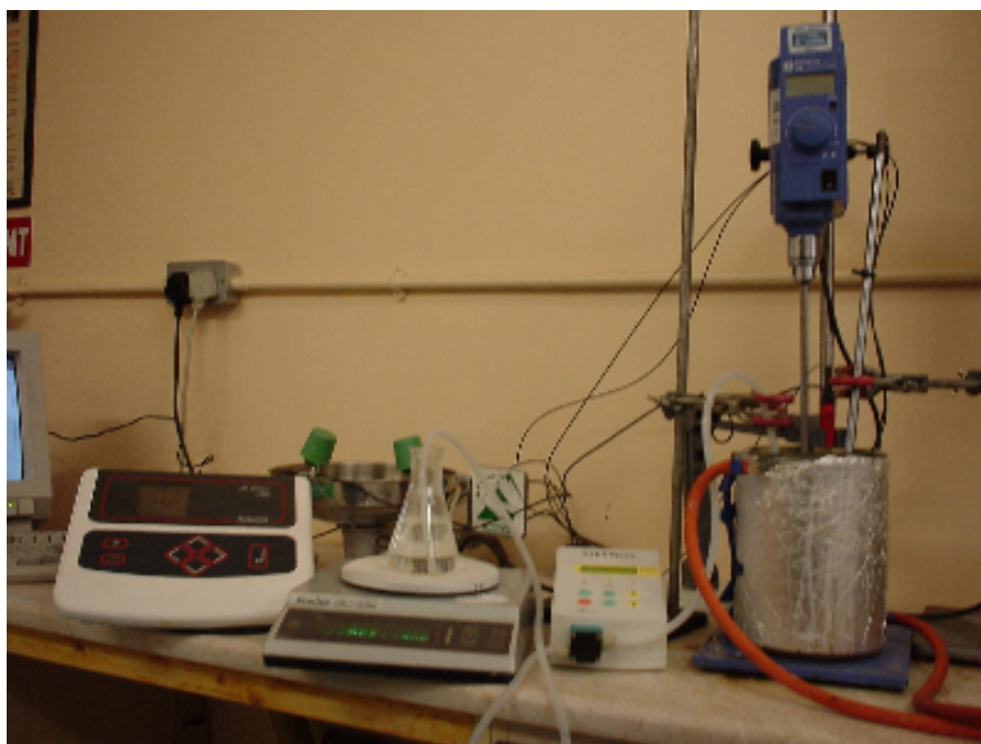
Figure 4.3 Agitation and acid addition rig shows jacketed vessel (bottom right), IKA stirrer motor (top right), HCl being added by peristaltic pump (centre) and Jenway pH and temperature meter (left).
