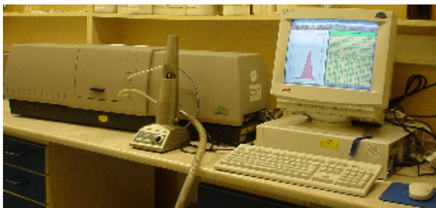
Figure 4.11 Malvern Mastersizer S optical unit connected to small volume sample presentation unit (pump) in front.
