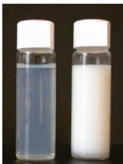
Figure 1.2 Picture of nanoemulsion (left) and conventional emulsion (right) with droplet diameters of 35 nm and 1 \mu\text{m} , respectively (Solans et al., 2005).
