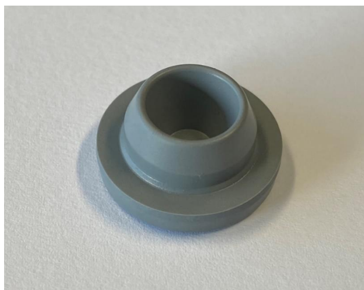
Figure S5.1: Schematic of uncoated, small volume bromobutyl stopper (A) and an image of an uncoated bromobutyl stopper used in this study (B).
