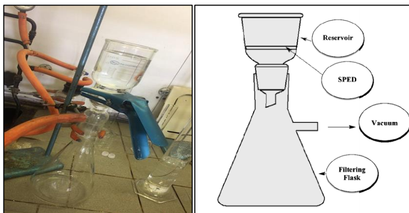
Figure 5.2 The setup for disk conditioning
