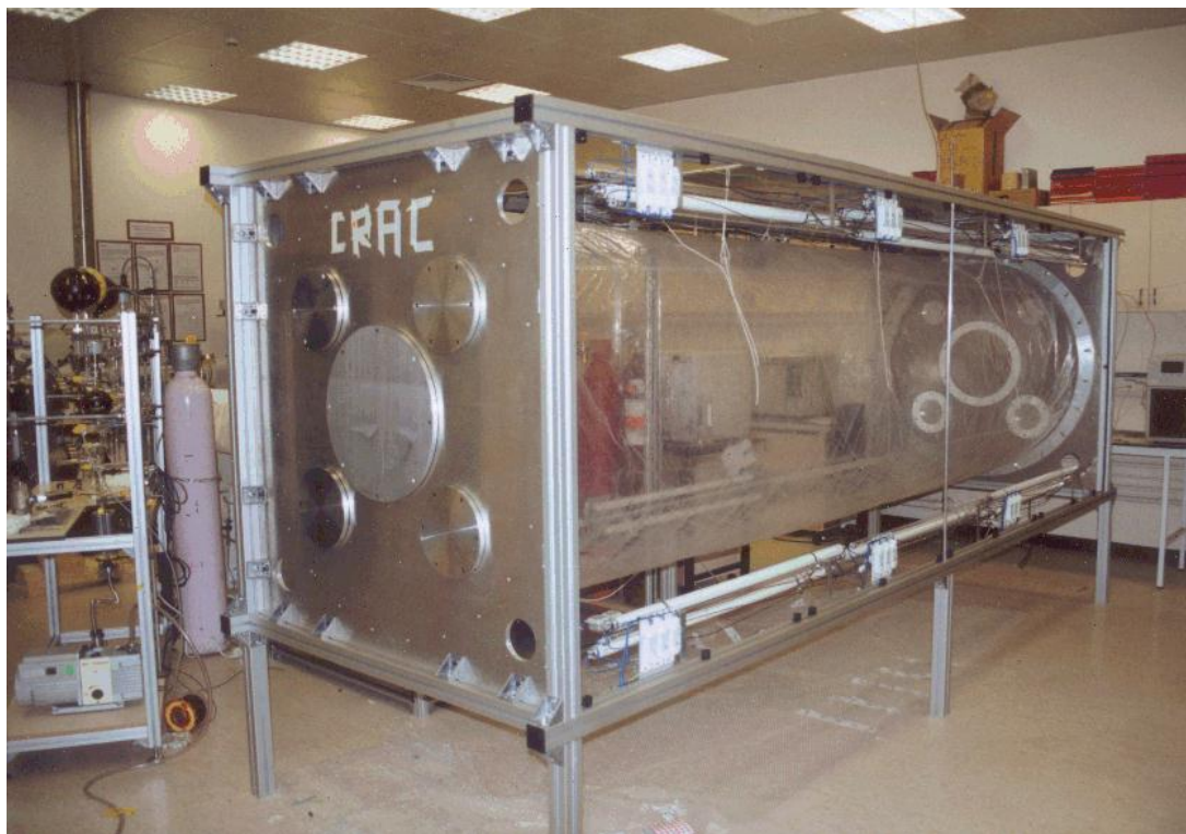
Figure 3.9 The 3.9 m 3 atmospheric simulation chamber at University College Cork.
