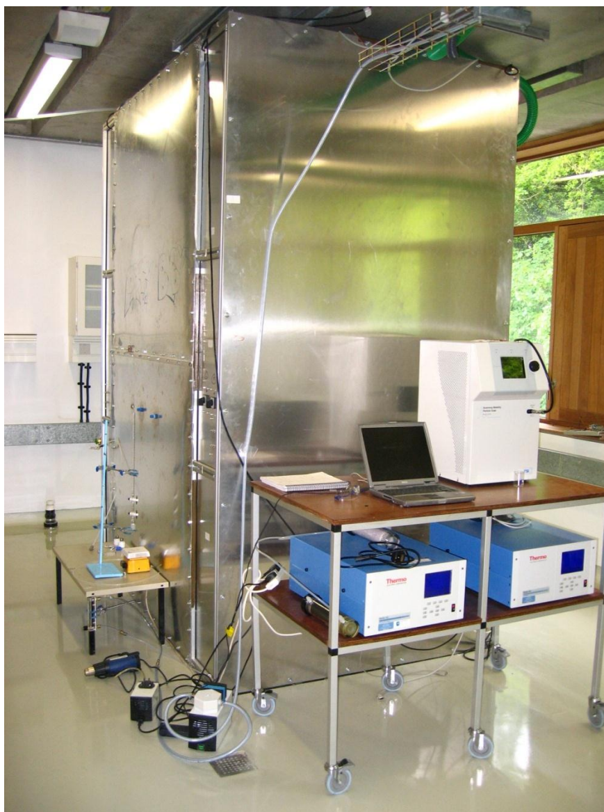
Figure 2.1 6.5 m 3 atmospheric simulation chamber in the Environmental Research Institute (ERI), University College Cork.
