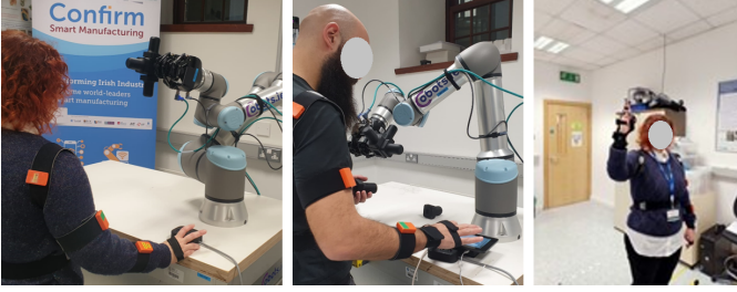
Fig. 6. Use of the three different HRIs during the 3D core tasks. From the left: the keypad, the touchscreen and the data glove.
