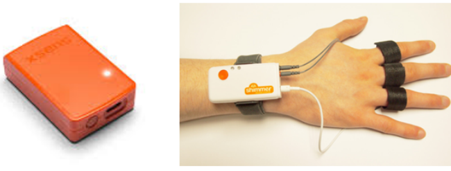
Fig. 2. Wearable sensing technologies used in the trust assessment. From the left: IMU, and GSR sensor.
