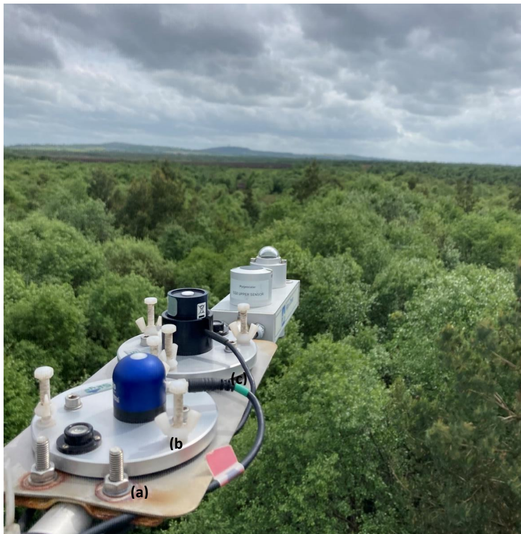
Figure 3.16 Radiation sensors mounted at the top of the EC tower (photo: author).
