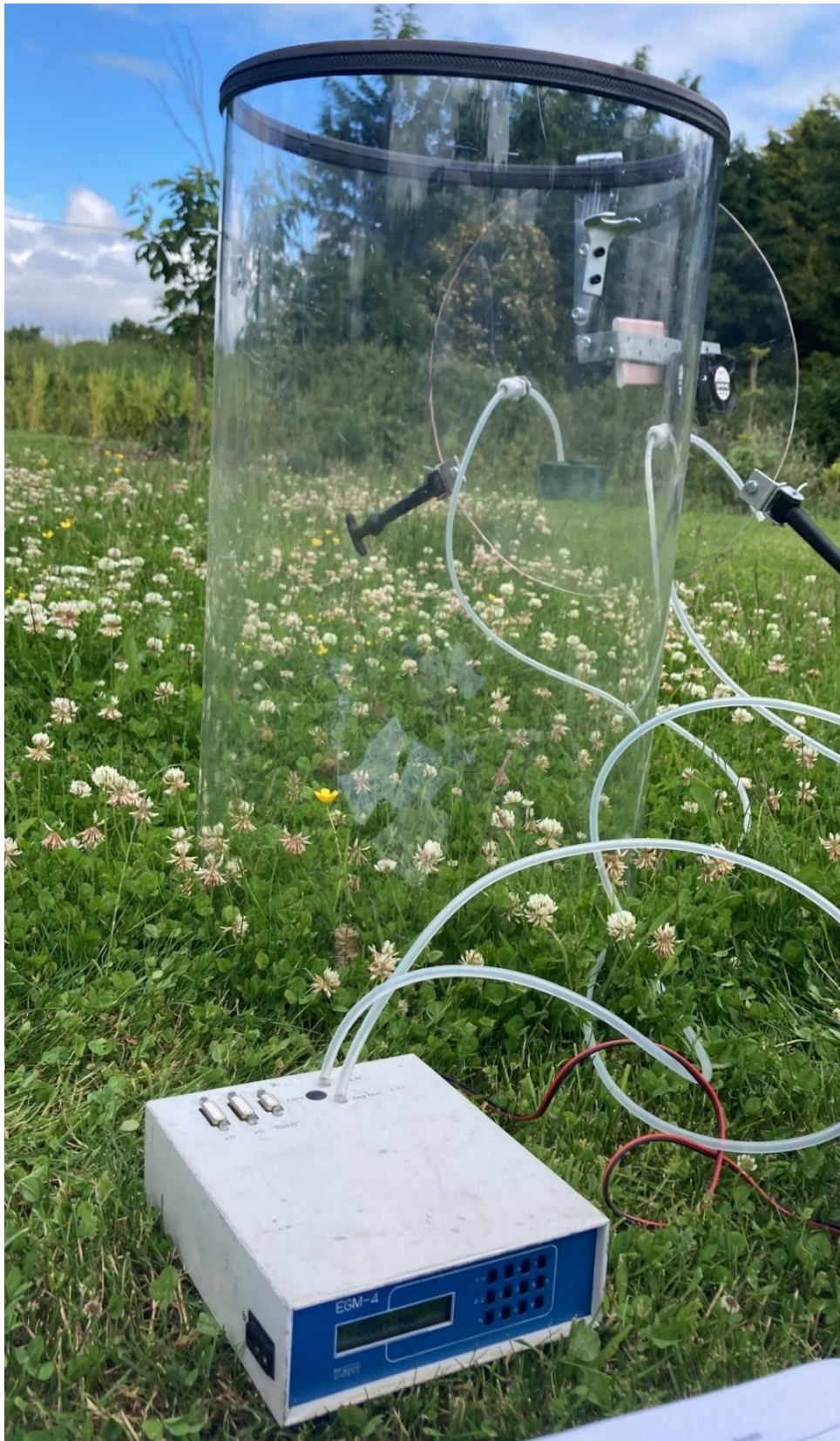
Figure 3.8 Clear static chamber connected to the EGM-4 analyser (photo: author).
