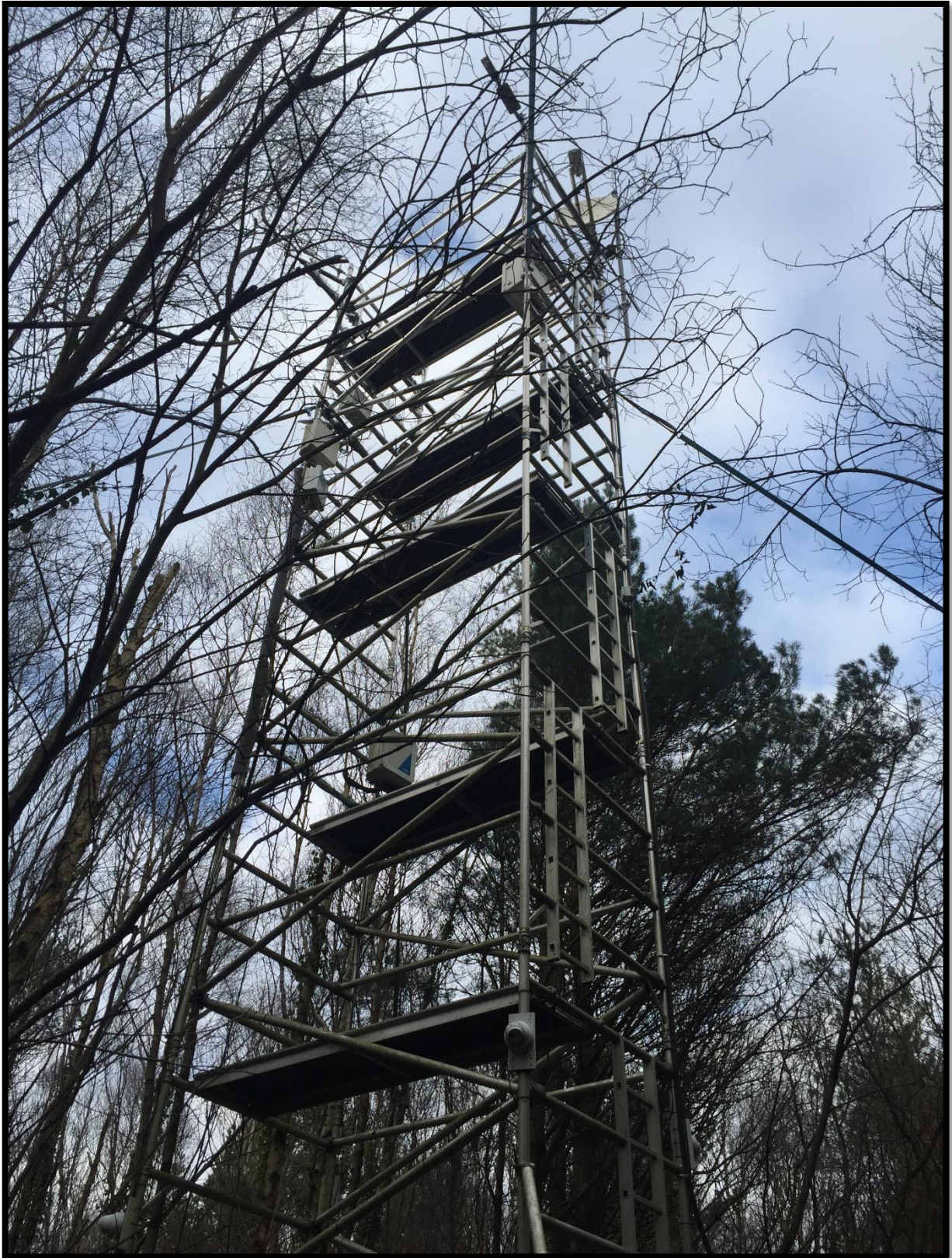
Figure 3.13 The eddy covariance tower at the Lullymore site (photo: author).
