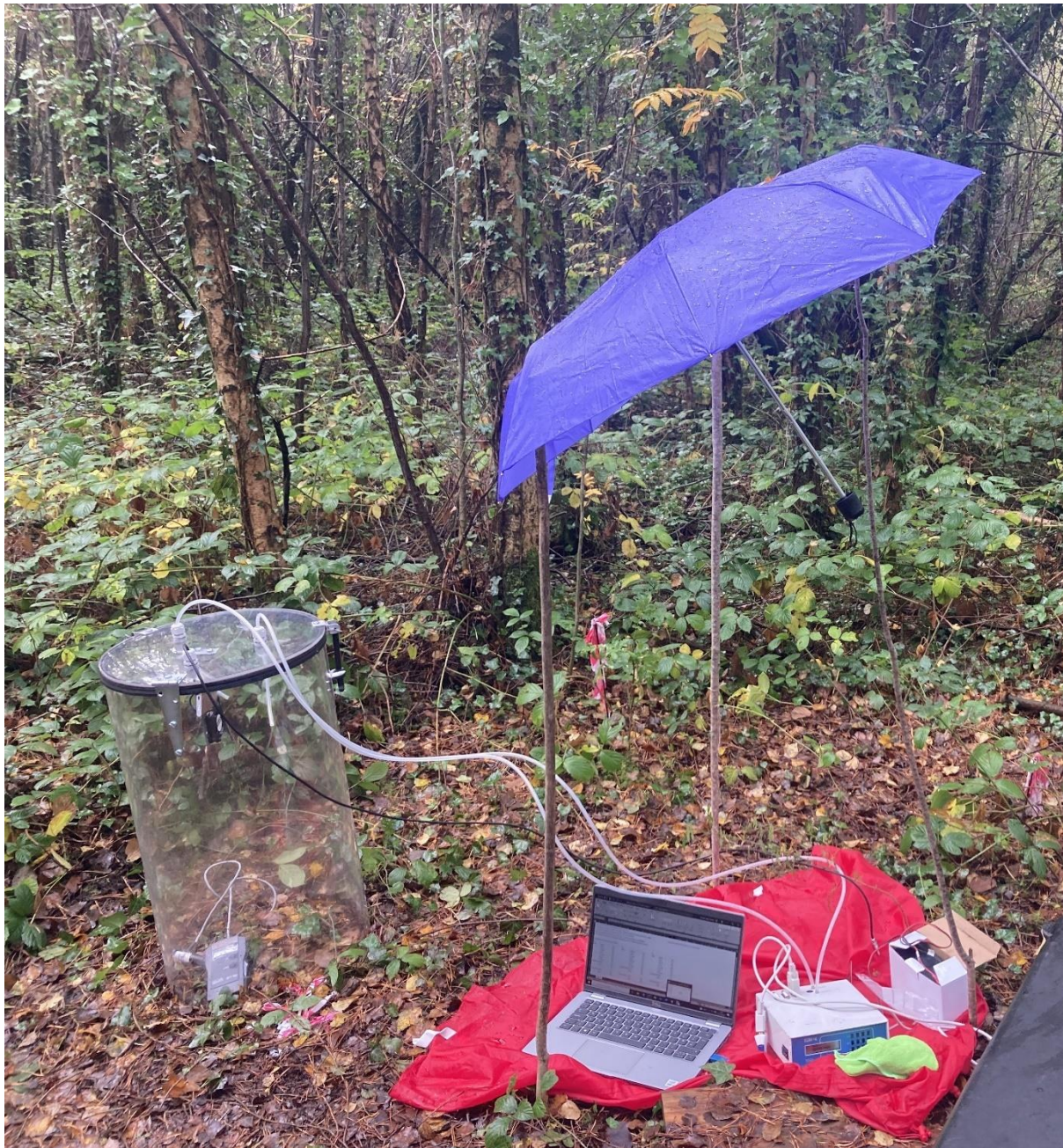
Figure 3.9 Below canopy chamber measurements at Lullymore taking an NEEbel measurement (photo: author).
