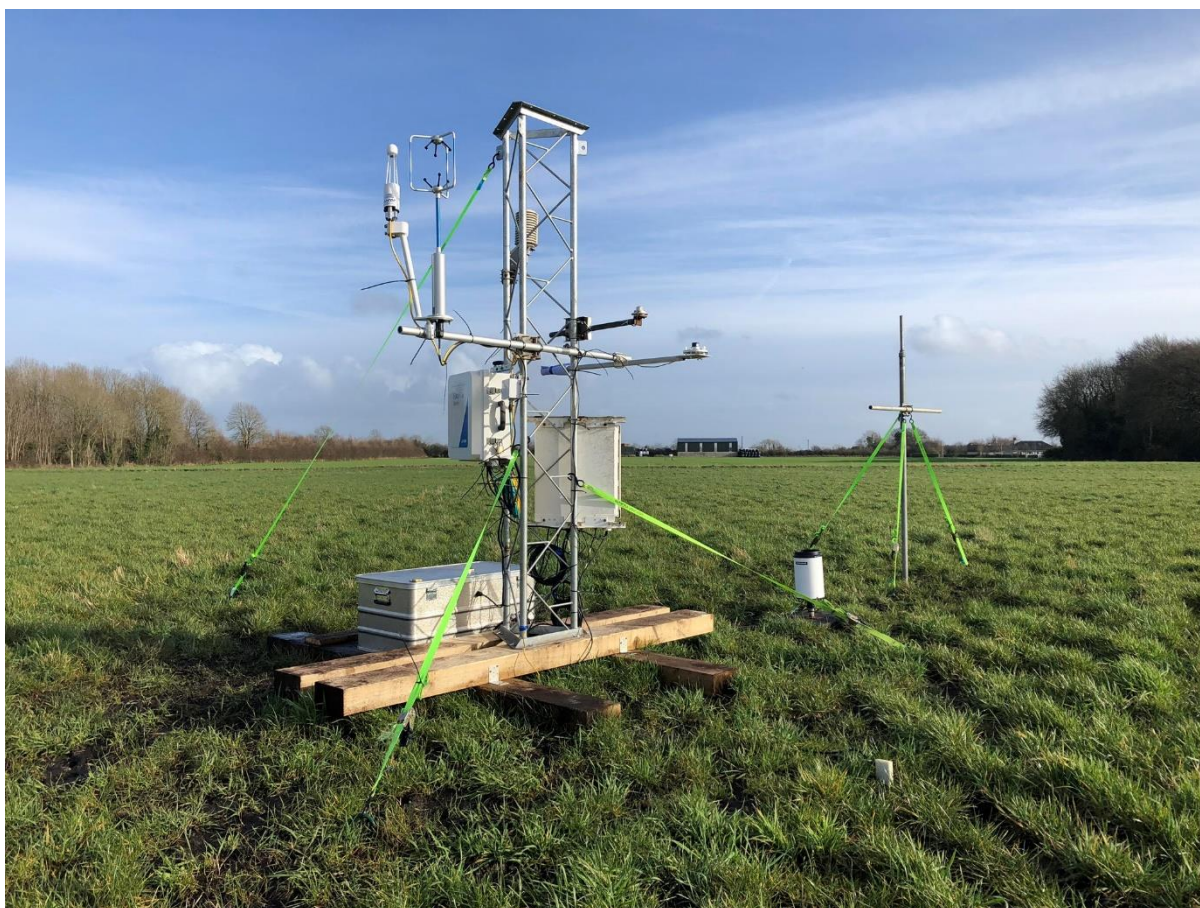
Figure 2.4 Eddy covariance system, monitoring CO 2 fluxes from a grassland on peat soils, located at Lullymore Kildare Ireland (photo: author).
