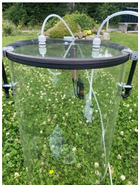
Figure 2.10 Static chamber made from translucent material intended to measure NEE & Respiration (photo: author).
