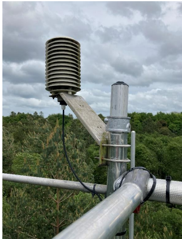
Figure 3.18 Humidity and temperature sensor positioned on top of EC tower (photos: author).
