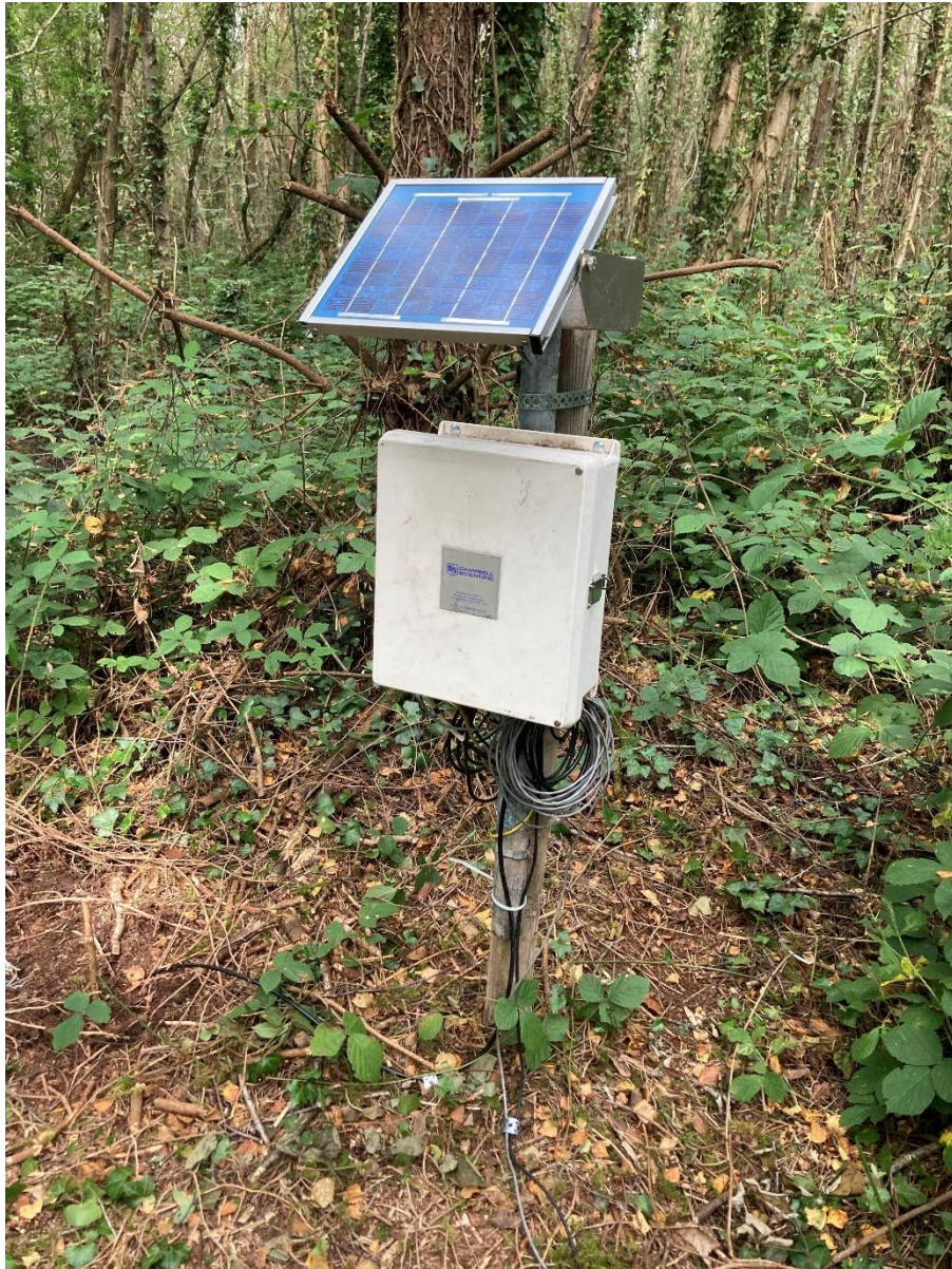
Figure 3.20 below canopy meteorological station containing the CR200 datalogger (photo: author).
