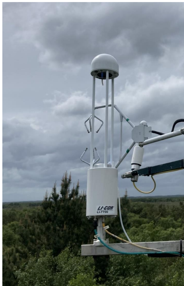
Figure 3.15 Li-Cor Li7700 open path CH 4 analyser (photo:author).
