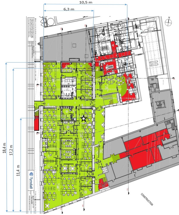
Figure 8. 868MHz range test
