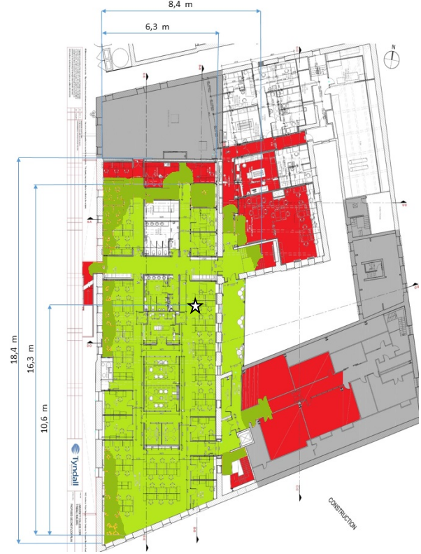
Figure 10. ZigBee 2.4GHz range test
