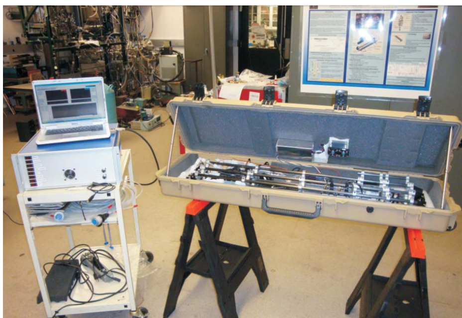
Figure 8-8: The earliest version of the new cage design that was employed in the NOxCaRD instrument in 2009.
