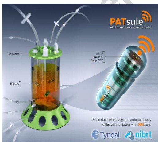
Fig 5 Concept of the PATsule technology and how it can be incorporated into a bioreactor
