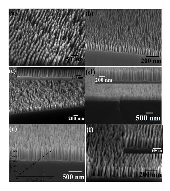
**Fig. 3** Cross sectional SEM images of Si nanopillars with different diameter and height (a) 21 nm, 50 nm, (b) 21 nm, 100 nm, (c) 21 nm, 150 nm, (d) 21nm, 400 nm, (e) 21 nm, 500 nm, (f) 27 nm, 150 nm and (f, inset) 15 nm, 150 nm respectively. Inset of (c, d) shows oriented Si nanopillars with 42 nm spacing between them. Inset of (e) shows the variation of nanopillar height with etching time.
