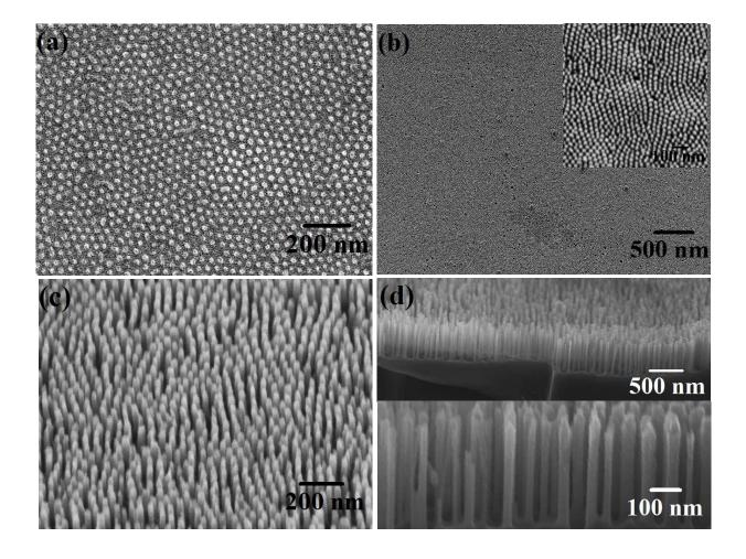
**Fig. 1** SEM images of (a) hexagonal ordered iron oxide nanodots on Si substrate, (b) nanopillar arrays with iron oxide nanodots at top formed after pattern transfer onto silicon, (c) Si nanopillars after removal of mask and (d) cross-sectional image of 500 nm long Si nanopillars. Insets of (b) and (d) shows corresponding higher magnification SEM images revealing the hexagonal arrangement.
