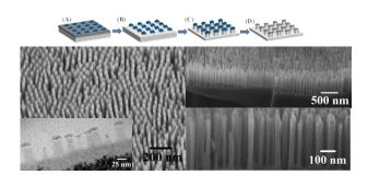
A novel, simple, cost effective and insitu hard mask technology is used to develop high aspect ratio silicon nanopillar and nanowire arrays over wafer scale. Iron oxide was found to be an excellent resistant mask over silicon. The nanopillars are crystalline with desirable uni-axial crystallographic orientation having uniform diameter and smooth sidewalls throughout their entire length. The aspect ratio of the nanopillars can be easily controlled.
