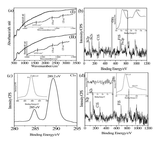
**Fig. 2** (a) FTIR absorption spectra of the etched sample before (I) and after (II) iron oxide removal. Insets shows corresponding spectra in 100-1300 cm<sup>-1</sup> range. XPS survey spectra of the nanopillars on Si substrate (b) before and (d) after removal of iron oxide. Insets of (b) and (d) shows corresponding high resolution Fe2p spectra. (c) and inset shows high resolution C1s and F1s spectra. Inset of (d)(right) illustrates Si 2p spectrum.
