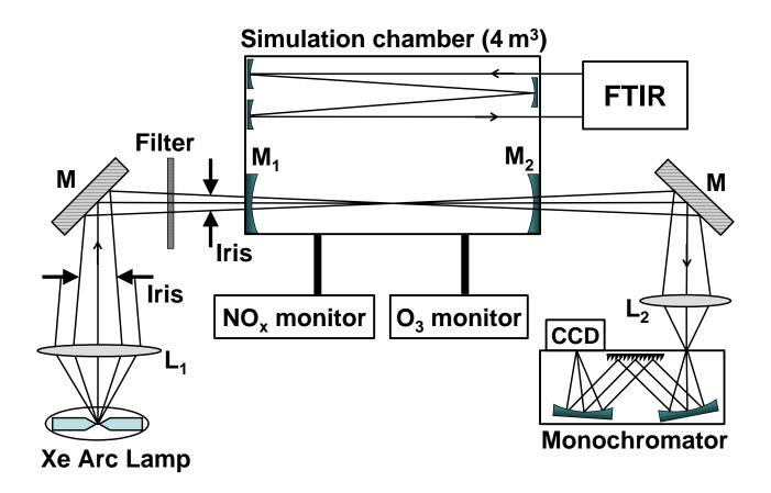
**FIGURE 1.** Schematic diagram of the experimental setup.  $L_1$  and  $L_2$ : lenses; M: metallic mirrors;  $M_1$  and  $M_2$ : high reflectivity dielectric mirrors with  $R \approx 0.99775$  at 665 nm; Filters: Schott RG 610 and RG 630 of 1mm and 3 mm, respectively; FTIR: Fourier Transform Infrared spectrometer.
