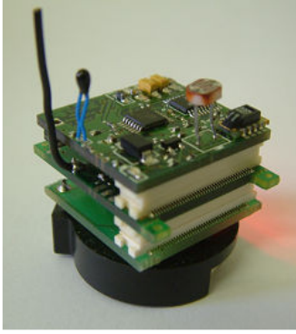
Figure 6. The Multisensor Layer in the modular stack
