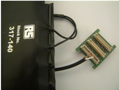
Figure 7. 25mm Generic Sensor Interface Layer connected to a pressure mat
