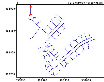
Fig. 2. European LV Test Feeder [23]
