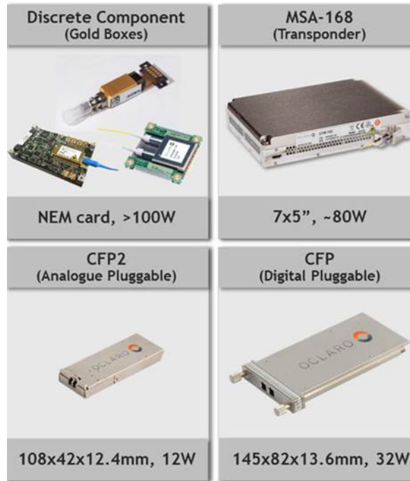
Figure 1.2: Dimensions and power requirements of C form-factor pluggables formats (CFP) for optical transceivers [19].
