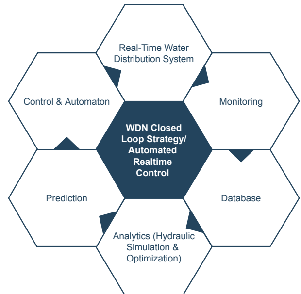
FIGURE 3. Closed-loop strategy for water supply system.
