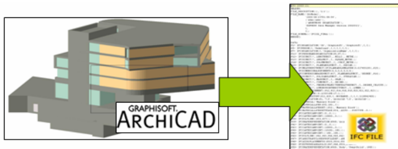
Figure 4-1 – Exporting a building generated in ArchiCAD as an IFC file
