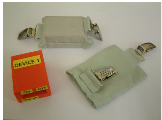
Figure 5. Cloth enclosure for WIMU ensuring the devices remain sterile while minimising artifact introduction.
