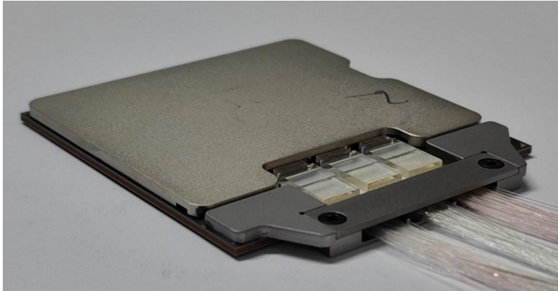
Figure 6: A fully packaged edge-coupled FPGA multichip package demonstrating three 56-channel FAUs attached to the MCP
