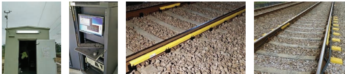
Fig. 4. Wayside system in Portugal: data processor unit and system installation in the track.
