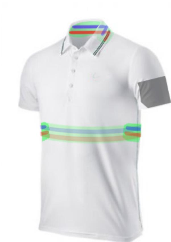
Figure 6.1: A conceptual image of a t-shirt that incorporates both the ECG and ICG systems via patches built into the shirt. A BP cuff could also be incorporated into the arm and a ring photoplethysmograph sensor could also be included.
