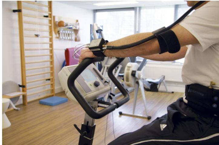
Figure 2.10: The Portapres Device being worn during an exercise test with the associated finger cuffs, their servo controller and 5kg belt. Image taken from Finapres website [85].
