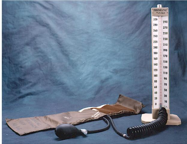
Figure 2.2: A “gold standard” mercury sphygmomanometer [22].
