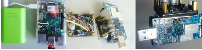
Figure 3. Left: A Pi with a Raspbee. Middle: An EPM device and a Tmote sky (attached with a metal plate). Right: the EPM holding a sensor node with its magnets.
