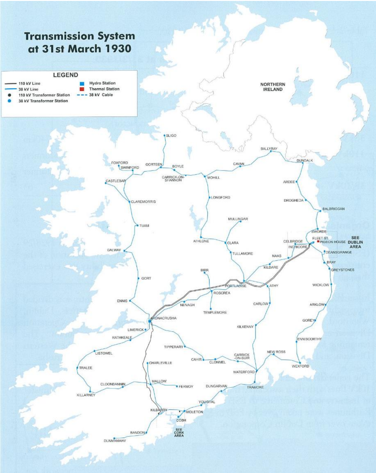
Figure 1: Ireland’s transmission system in 1930
